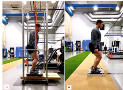
Figure 1. (A) Isometric Mid-Thigh Pull (IMTP) Rig; (B) Dual-Handle Portable (DHP) Rig
